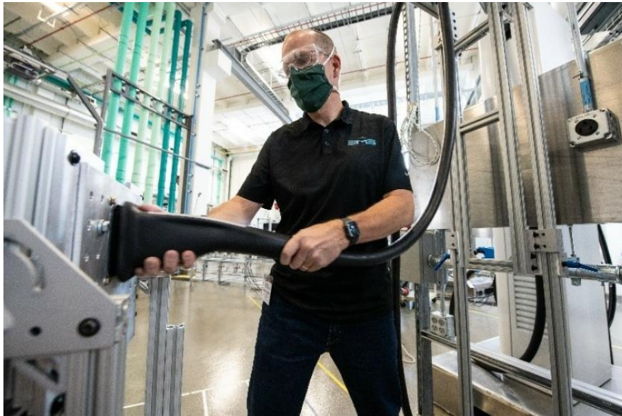
Figure 5 MCS Connector testing at NREL facilities 9
